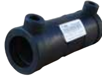
EF COUPLER (LONG) EF MANŞON (UZUN) SDR 11 PE100 GAS / GAZ : 10 BAR WATER / SU : 16 BAR
